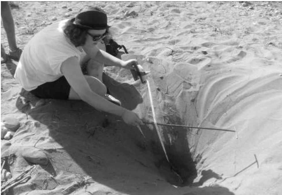
Figure 5: Measuring the depth of the position of the Tiny Tag
