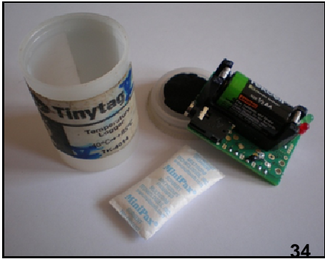
Fig. 34: Tinytag with PVC-film canister
