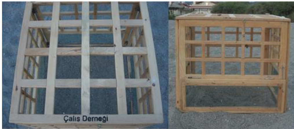
Figure 1. Wooden protection cage top view (left) and front view (right), used for experiment for potential future Caretta caretta nest protection at Calis Beach (photo: M. Lambropoulos)
